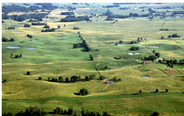
Fig. 2. Variation in karst terrain. (a) Mountain karst in Sichuan, China, with bare rock on the hillsides and soil floors within isolated depressions. (b) A lowland plain in Kentucky, USA, with numerous sinkholes in a soil cover that overlies cavernous limestone.
